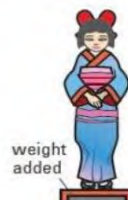
Figure 5.25c centre of gravity lowered by adding lead to base
